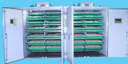
SETTER INCUBATOR INTERIOR CAPACITY 30,240 EGGS
